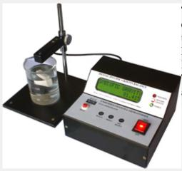
This is the ESLPL® most popular yet simplest to use, accurate and economic model of digital specific gravity balance which can be used to test specific gravity of solid materials like Rubber, PVC, Plastic, Metal, Wood etc. Being load cell as a base of measurements It covers a wide range of specific gravity which goes 0.01 to 22.000. The weight sample should be in between 2 grams to 50 grams in air as well as in water.
